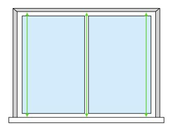
Measure in 3 places across the width of the window - The smallest measurement will be your width. Then measure in 3 places down the height of your window - The smallest measurement will be your drop.
